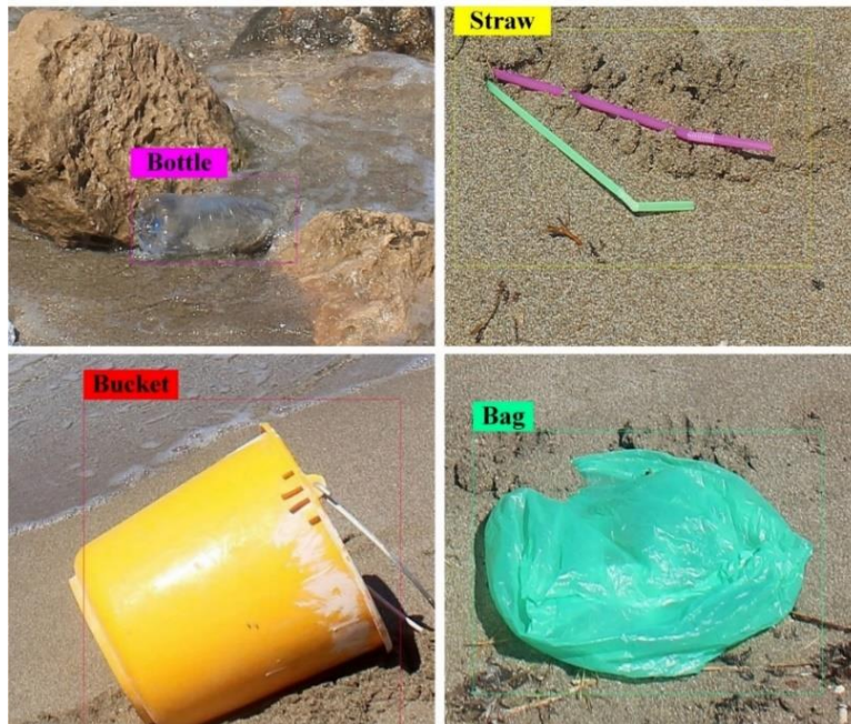
Figure 36: Examples of correctly recognised plastic litter articles obtained from the YOLOv4 object detector.
