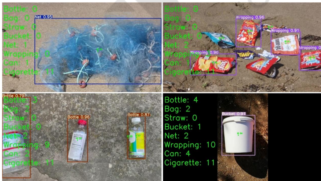
Figure 48: Screenshots demonstrating the application of the YOLOv5 object detector and the centroid tracking method on an actual field video.
