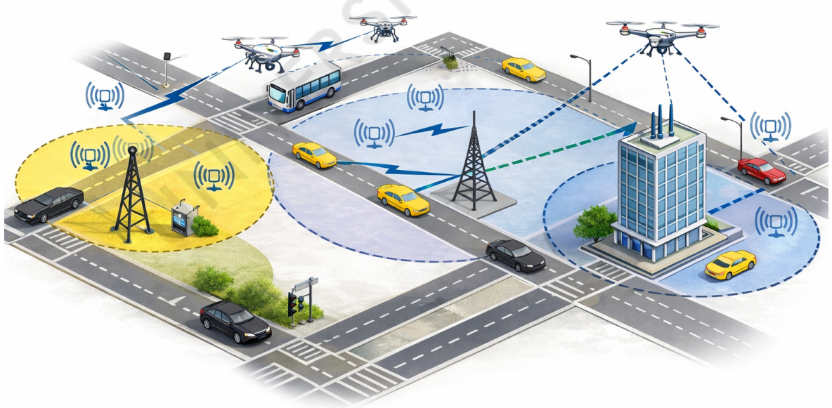
Figure 2.8: Ad-hoc multi-agent communication scenario involving UAVs, vehicles, and terrestrial infrastructure.
