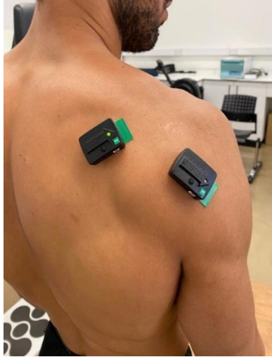
Figure 4.2. The EMG electrodes placement for the INF muscle and PD muscle.
